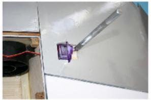
Trial fit he servo. Cautiously make a small incision through the top covering. This is where slot of the control-horn will be cut.
