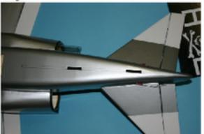
Now it is time to install the vertical fin. Mark the outline of the fin on the fuselage. Carefully trim the marked covering with some inner offset.
