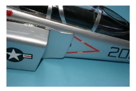
Glue the inlet streamers" to the fuselage in front of the intakes. Note there's a cooling slot just in front of the inlet streamer.
