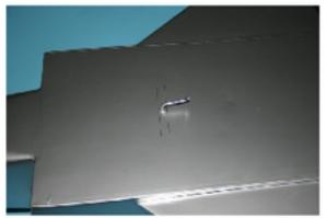
Inside the fuselage just in front of the bulk head located between the wing root tips a hard wood block is glued. Locate the hard wood block and drill a 2mm hole for the bungee hook . glue the bungee hook in the fuselage.
