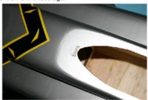
Now you can glue in one of the supplied magnets in the fuselage. Cut out a slot for the magnet and glue the magnet in this slot.
