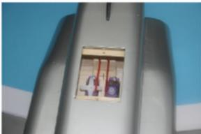
Glue the tray underneath the top-hatch on the turtle deck floor (above the fan units).
