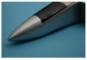
Now you can glue on the fibreglass nose and the exhaust dummies. To make the plane more appealing you can spray paint the nose white before you glue it to the fuselage see the picture. All these fibreglass parts can be glued with 5 minute epoxy.
