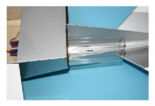
Fit the tube to the fanunit. (read fanuit installation instructions first) You should have installed the motor and ESC already. Make a hole for the wires from the esc and route them trough the just made hole.. Now take of the tube and insert it from the back by squeezing the tube a little. Leave enough room to install the fanunit.
