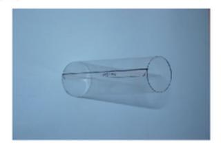
Cut out the unrolled surface for both trust tubes. Put the ovelap area inside. Roll the pvc to a tube and apply outside adhesive tape. The Edge should match the innerline of the overlap area. Now you have a perfect conical trust tube.
