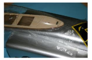
Before you glue the canopy to the canopy floor put some plastic film (cut open thin plastic bag) underneath the cockpit floor and slide in onto the fuselage. This prevents that the removable canopy will be fixed forever to the fuselage.
