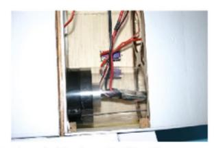
Now install the fanunit. Chamfer the front of the shroud of the fanunit a little with a sharp knife this will make it eassier to install the fanunit inside the duct. Now route the esc wires trhrough the hole in the trust tube you made.. And slide the Trust tube over the back end from the shroud. Use adhesive tape to attach the trust tube to the fan shroud.
