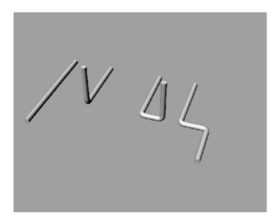
This picture shows the steps how to make a Z-bend. Steps are from left to right. You need 2 ordinary pliers. Practice first on a scrap steel rod.
