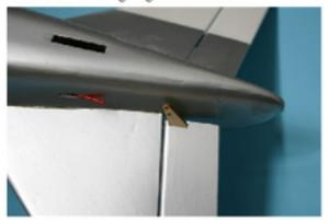
Cut the slots for the Bowden tube on both sides at the fuselage end as in the picture Wait before you glue the elevator control-horn in place, first make the pushrod. Make one Z-bend first (servo side) and insert the pushrod in the Bowden tube. Do this for both elevator halves.
