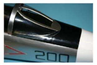
Now you can glue the small parabolic shaped piece of plywood in place. This piece is also glued on the bottom side of the canopy floor and should fit in the canopy opening, this parabolic shaped piece of ply wood prevents that the canopy moves back- or sideward during flight.
